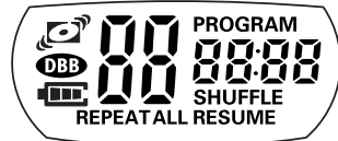
test pattern 1 (all segments activated)
